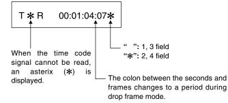
The control signals, time code, etc. are displayed using abbreviations.
